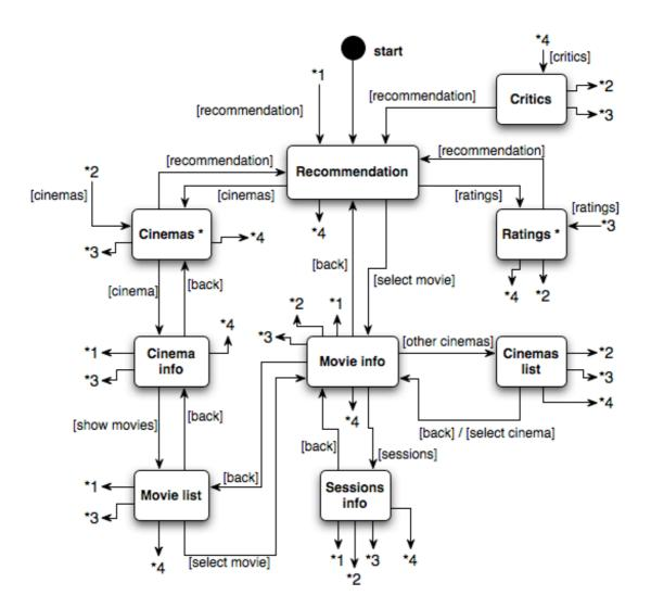
Figure 58. State diagram of the interface
