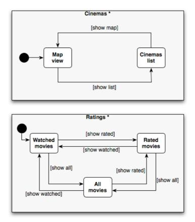
Figure 59. Super states of the state diagram (Figure XX)
